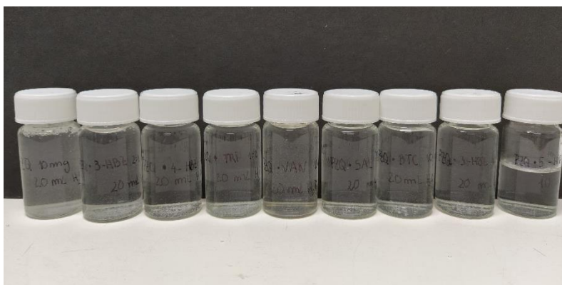
Figure 38 Solubility comparison for PZQ, PZQ·3-HBZ 2:1, PZQ·4-HBZ, PZQ·TRI 1:2, PZQ·VAN, PZQ·SAL, PZQ·BTC 2:1, PZQ·3-HBZ 1:1 and PZQ·5-HIP (from left to right).
